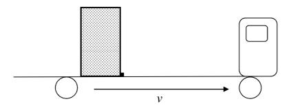
a) On the right of the block sketched in figure 3, sketch in the model block at the moment of toppling over. Mark on the centre of gravity. When it is at the point of toppling, what energy change has taken place?
