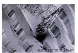
Stylus needle in a groove
