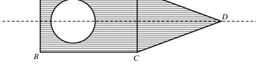
The figure above shows a uniform lamina ABCDE, formed by combining a rectangle ABCE and a triangle ECD. A circular disc of radius 4 cm is removed from the rectangle, so that the resulting lamina has a single line of symmetry. The centre of the disc is 6 cm from AB. The triangle ECD is isosceles with ED = CD. It is also given that BC = 17 cm and AB = 10 cm.
