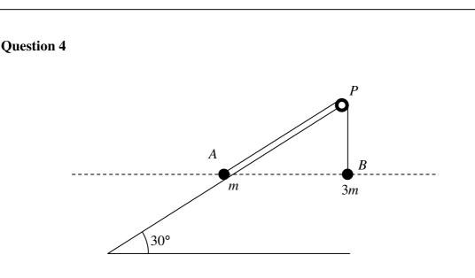
Two particles A and B, of mass m and 3m respectively, are attached to each of the ends of a light inextensible string. The string passes over a smooth pulley P, at the top of a fixed smooth plane, inclined at  $30^{\circ}$  to the horizontal.
