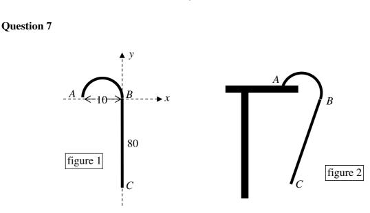
Figure 1 shows a walking stick ABC, modelled as two uniform rods AB and BC. The straight section BC has length 80 cm and the section AB is a circular arc of diameter 10 cm. The semi-circular section of the walking stick is **four times** as dense as the straight section. A set of coordinate axes is defined with B as the origin as shown in figure 1.
