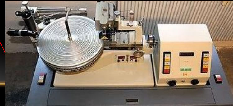
Disc Cutting Lathe- cuts metal master
