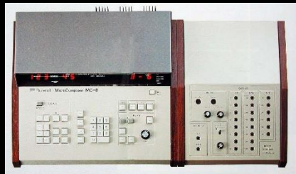
Roland MC-8 Microcomposer 1977, the first microprocessor-based digital sequencer
