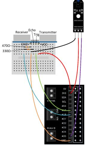
Push the ultrasonic sensor into the holes on the breadboard, with the pin marked GND in the same column as the jumper wire that goes to the ground of the EduKit Controller Board.
