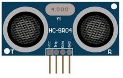
The HR-SC04 Ultrasonic Sensor module is used to detect the distance from the sensor to a surface.
