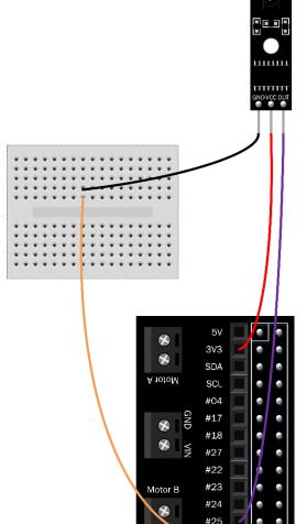
Use the three female-male jumper wires for all of the connections between the line follower and the motor controller board and breadboard. The male-male jumper connects between the ground of the controller board and the breadboard.
