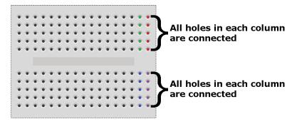
The breadboard is a way of connecting electronic components to each other without having to solder them together. They are often used to test a circuit design before creating a Printed Circuit Board (PCB).
