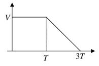
For the graph above, the time for the whole journey is 45 seconds. The acceleration between T and 3T is -1.5ms<sup>-2</sup>. Find
