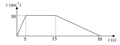
9. The total distance travelled during the motion shown in the velocity-time graph below is 900 m. Use this information and the graph to find V.
