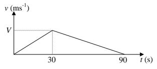
10. In the motion shown in the graph below, the initial acceleration is 2 ms<sup>-2</sup>.
