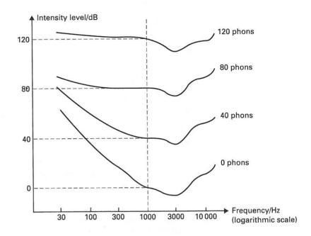
Another way of taking account of the <u>frequency</u> dependence of loudness is to use a sound level meter calibrated on a scale known as the **dBA scale**. The meter is essentially a microphone coupled to electronic circuitry that suppresses certain frequencies in such a way that the response of the microphone mimics that of a normal ear.
