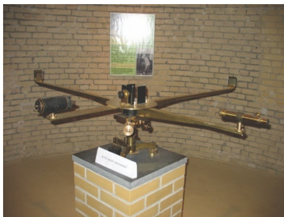
Figure 16.38 A Michelson–Morley interferometer. Although this apparatus is shown on a brick pillar, in the original experiment the interferometer took place in the basement of the laboratory. It was also placed on a heavy stone slab floating on a bath of mercury. This was to prevent any vibrations from affecting the measurements.
