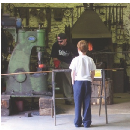
Figure 16.25 Blacksmiths can tell the temperature of the metal by observing its colour. Visible and infrared radiation are being emitted from the surface.
