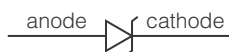
Figure 18.17 Circuit symbol for a Zener diode with the cathode and anode identified.
