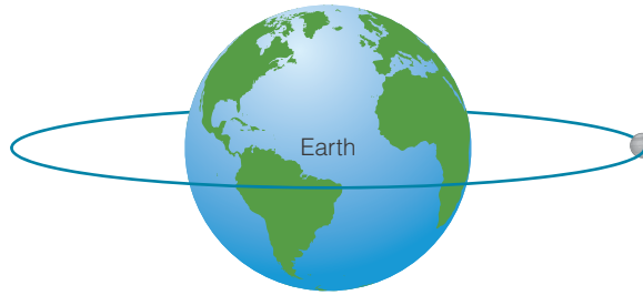
Figure 18.76 Geostationary or geosynchronous satellites are positioned above the equator.
