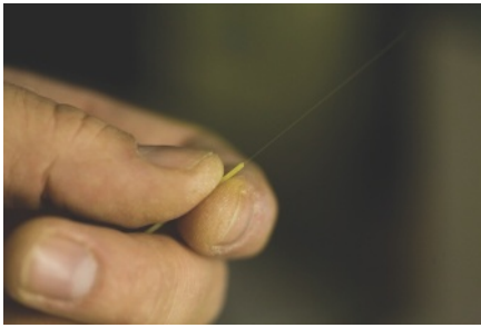
Figure 18.71 A fibre optic cable that can carry many thousands of telephone calls is much smaller than the equivalent copper cables.
