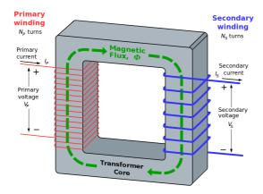
They consist of a primary and secondary coil of wire wrapped around a soft iron core. Both primary and secondary coils of wire are coated in electrically insulating material.
