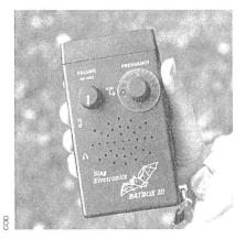
Electronic devices, such as the bat detector pictured above, can be used to estimate population density of nocturnal, highly mobile species, such as bats. In this case, the detector is tuned to the particular frequency of the hunting clicks emitted by specific bat species. The number of calls recorded per unit time can be
