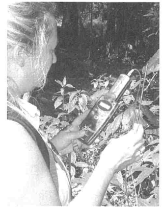
Dataloggers fitted with sensors are portable and easy to use in a wide range of aquatic (left) and terrestrial (right) environments. Different variables can be measured by changing the sensor attached to the logger.
