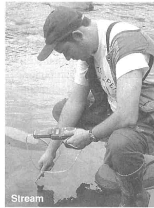
Dataloggers fitted with sensors are portable and easy to use in a wide range of aquatic (left) and terrestrial (right) environments. Different variables can be measured by changing the sensor attached to the logger.
