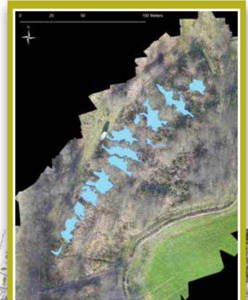
Unmanned Aerial Vehicles (UAVs) were used to create high resolution maps of the site, and identify standing water.
