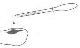
(c) **Porosity** The above test can be quantified by older children. Weigh the rocks dry, then immerse them in water. Bubbles can be seen as air from the pores in the rocks comes out. Leave for about 5 minutes. Which rock absorbs most water? Pat the rocks dry and weigh them again. The most porous rocks will have the largest weight gain.
