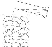
(h) Acidity Older children may test for this by adding distilled water to the soil, shaking then filtering the water off. This is then tested with Universal Indicator solution or papers. Commercial kits can be easily bought from garden centres or school suppliers. It can be a difficult test to get clear results, so it is a good idea to test the soil before letting the children do it.
