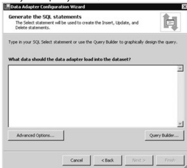
Figure 16-5: The screen to specify the SQL statement when the Use SQL statements option is selected
