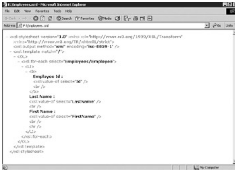
Figure 30-3: The Employees.xml file as displayed in the browser after including an XSLT style sheet
