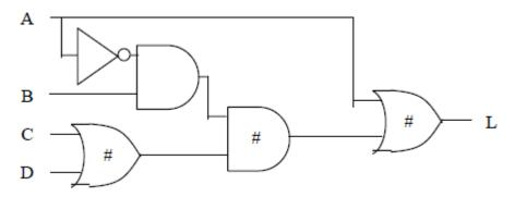
Solution 4 (solution 2 plus check for A off):
