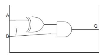
Inputs A and B connected to an XOR gate;
