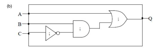
1 mark for NOT gate correctly linked to input C;
