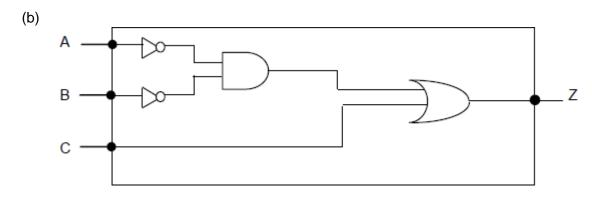
1 mark for NOT gates on both A and B; 1 mark for AND with inputs from  $\overline{\overline{\bf A}}$  and  $\overline{\overline{\bf B}}$ ;
