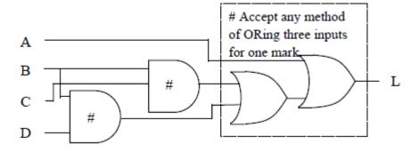
Solution 3 (solution 1 plus check for A off):
