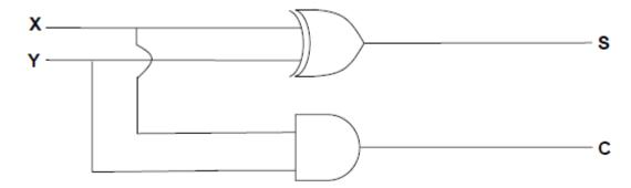
(i) Complete the truth table below for the logic circuit in the diagram above.
