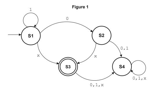
Input strings of 0x and 1x are accepted by this FSM.
