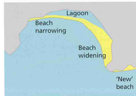
Figure 4 Longshore sand transport moving sand alongshore from west to east causes erosion and beach narrowing at the western end and accretion and beach widening at the eastern end
