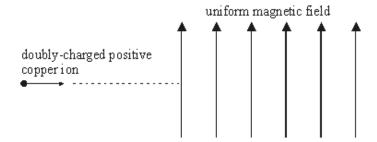
The diagram above shows a doubly-charged positive ion of the copper isotope  $^{63}_{29}$  Cu that is projected into a vertical magnetic field of flux density 0.28 T, with the field directed upwards. The ion enters the field at a speed of 7.8 × 10<sup>5</sup> m s<sup>-1</sup>.
