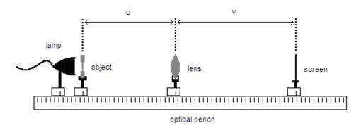
Adjust the position of the components until a focussed image of the grid is formed on the screen. Note that it will not be possible to form a 'real' image on the screen if the object distance is less than the focal length of the lens.
