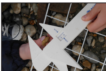
Figure 4. One way of measuring the long-axis of a beach pebble, using a stone calliper
