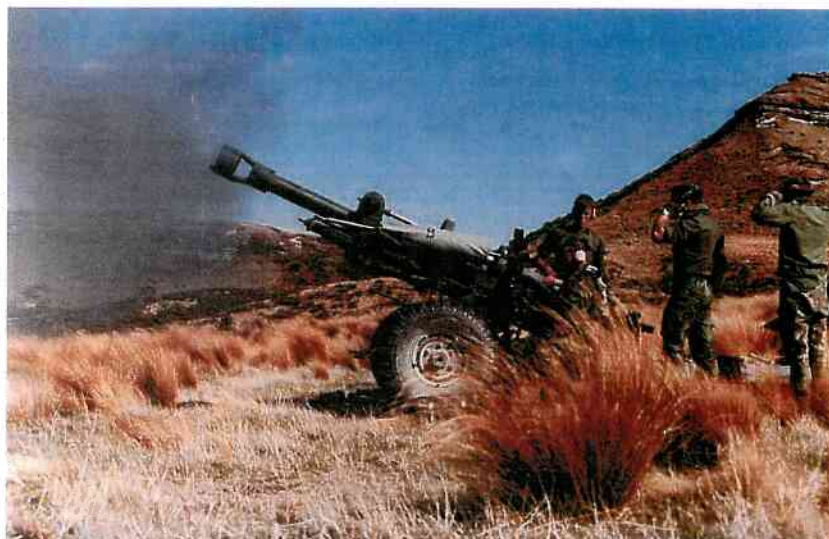
Figure 1 The gun barrel recoils when the shell is fired. Large springs fitted to the barrel take away and store the kinetic energy of the barrel as it recoils
