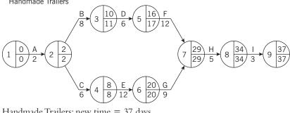
Handmade Trailers: new time = 37 days Critical path: A; C; E; G; H; I Total float: (29 - 12 - 16) = 1 hour
