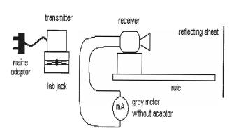
The standing waves experiment requires a board to reflect the microwaves back upon themselves. You should find a variation in intensity recorded as you move the receiver slowly along the line between the transmitter and the sheet. Note you will not obtain complete cancellation in the standing wave pattern. Measure the total distance over several maxima and minima, and use this to calculate the average distance between successive maxima or minima.
