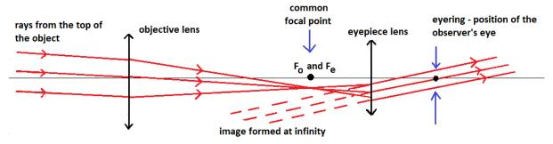
2. (a) 'normal adjustment' is when the telescope has been adjusted so that the virtual image seen by the observer is at infinity
