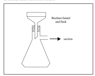
A small amount of cold solvent should be used to wet the filter paper prior to filtration, and to remove any solid remains from the reaction flask.
