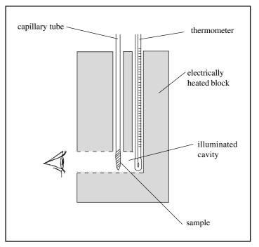
The sample is placed in a capillary tube, and the temperature increased slowly until it melts.
