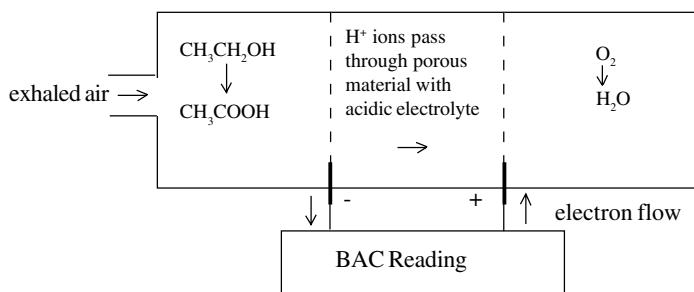
If the exhaled air contains ethanol (the fuel), the ethanol is oxidised at the platinum anode (negative) to ethanoic acid, hydrogen ions and electrons.
