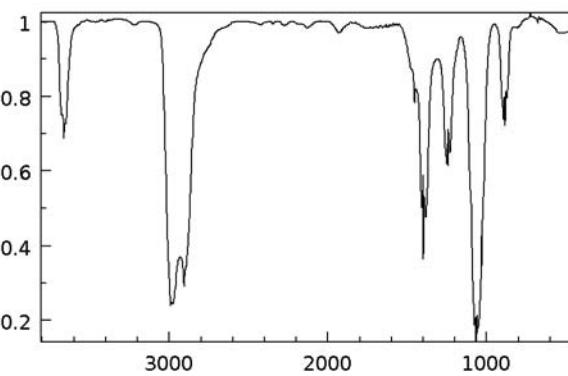
The ethanol concentration in a person's breath is determined by measuring the intensity of the absorption band at  $2950\text{ cm}^{-1}$ . The person's breath also contains water vapour which has several strong IR absorptions including bands at about  $3600\text{ cm}^{-1}$  and  $3800\text{ cm}^{-1}$ .
