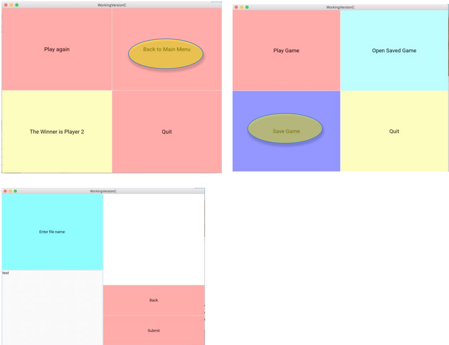
Fig 10.8 Transitioned from winner screen to main menu screen, but game can be saved when it shouldn't be able to- game is completed.
