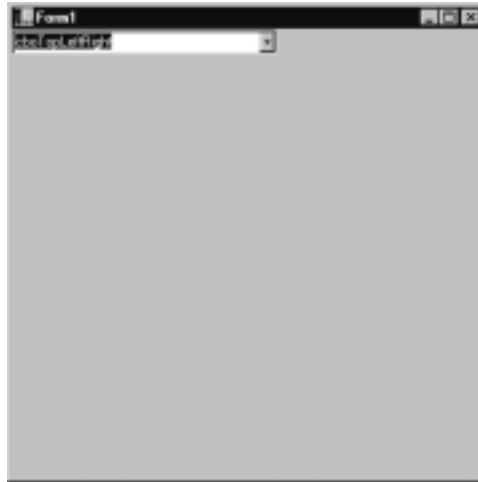
Figure 7.3 The Combo Box Anchored to the Top, Left, and Right Edges of a Form after Resizing
