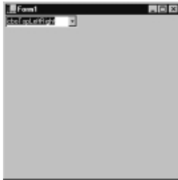
Figure 7.2 A Combo Box Anchored to the Top, Left, and Right Edges of a Form
