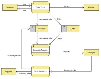
The Food Order System Data Flow Diagram example contains three processes, four external entities and two data stores.
