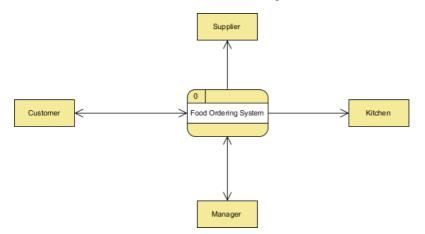
Context DFD is the entrance of a data flow model. It contains one and only one process and does not show any data store.
