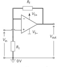
$$Gain = \frac{V_{out}}{V_{in}} = 1 + \frac{R_f}{R_1}$$
