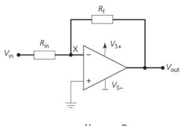
$$Gain = \frac{V_{out}}{V_{in}} = -\frac{R_f}{R_{in}}$$
