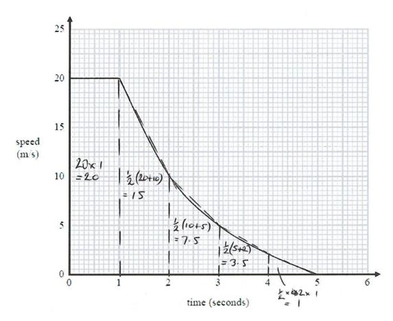
(a) Work out an estimate for the distance the car travels in these 5 seconds.
