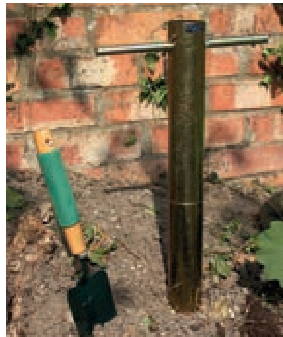
▲ A soil auger collects a more standardised sample than a trowel
