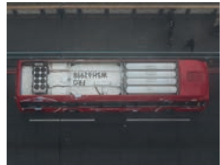
▲ A hydrogen fuel cell bus with storage tanks on the roof
