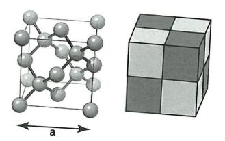
The length of the cube is **a** pm (1 pm =  $1 \times 10^{-12}$  m). The total number of silicon atoms contained within the cube is denoted **n**. The single crystal was fashioned into a perfect sphere of volume **V** cm<sup>3</sup>, and mass **m** g. The relative atomic mass of silicon is **A**<sub>r</sub>.
